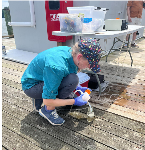
Figure 3: Amanda Reynolds demonstrates discrete water sample collection.
